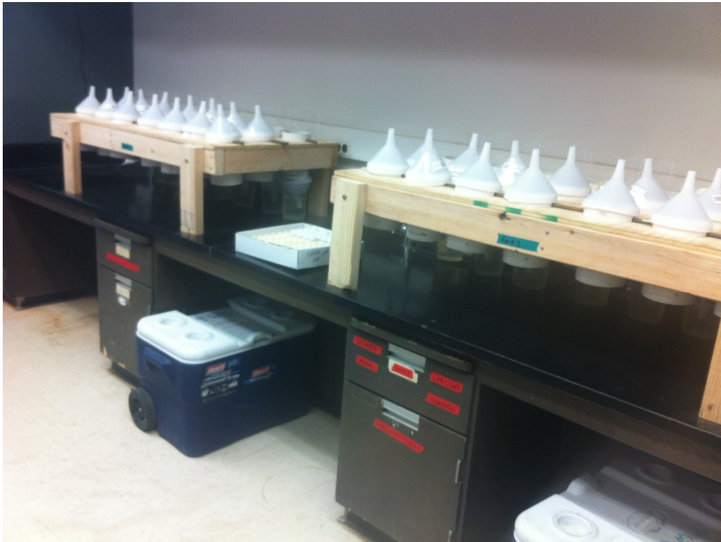
Figure 5. Replicates 3 & 4 on benchtop in laboratory with funnels placed on top of columns in between leaching events.
