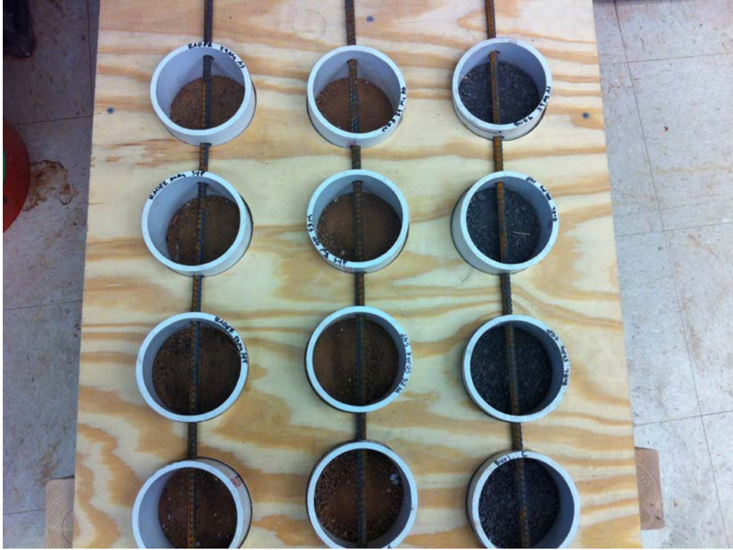
Figure 4. Experimental unit replicate setup containing a total of 21 columns of 3 soils x 7 fertilizer treatments.
